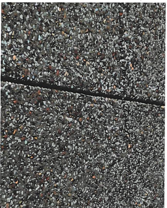
EXPOSED AGGREGATE CONCRETE PAVING (ALTERNATE)
